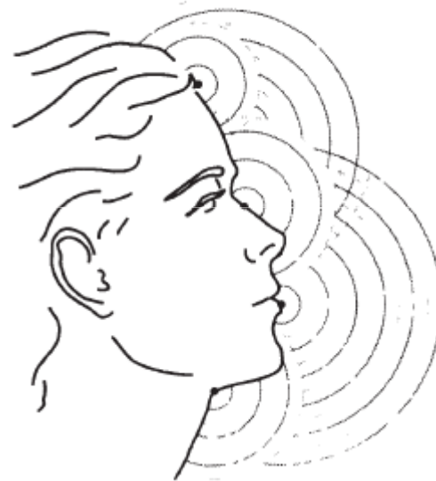
Figure 5.2 A person's face, like everything else we ordinarily see in reflected light, is covered with countless atomic scatterers.
